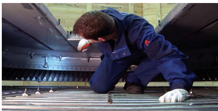
Figure 8. Ergonomic and safe inspection of a Torus™ quench section
